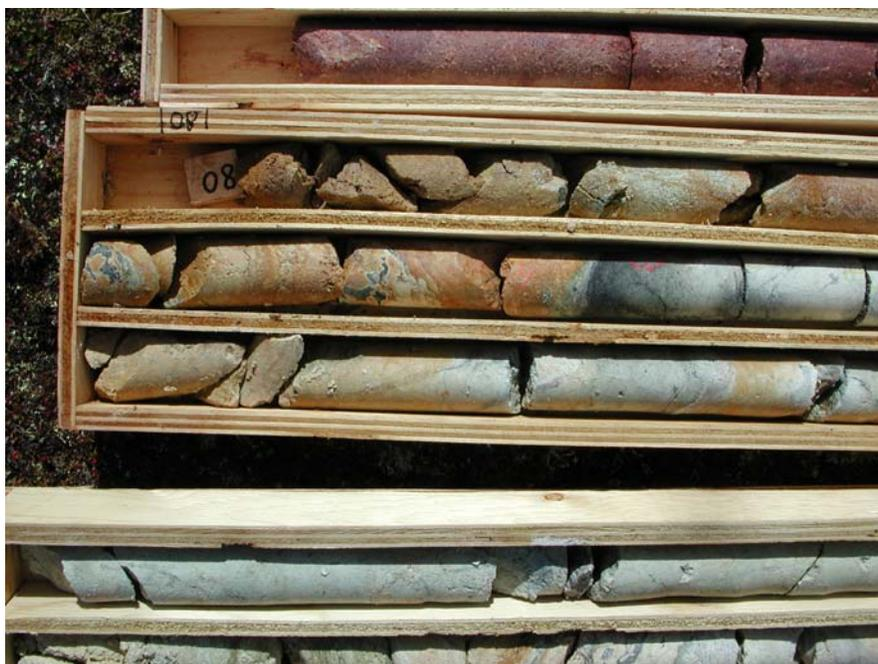
Illustration 1: Drill core from the Kiggavik deposit, Nunavut, illustrating the gradation from hematite alteration (red) through bleach clay alteration (biege) to deposition of uraninite (a uranium mineral, black).
