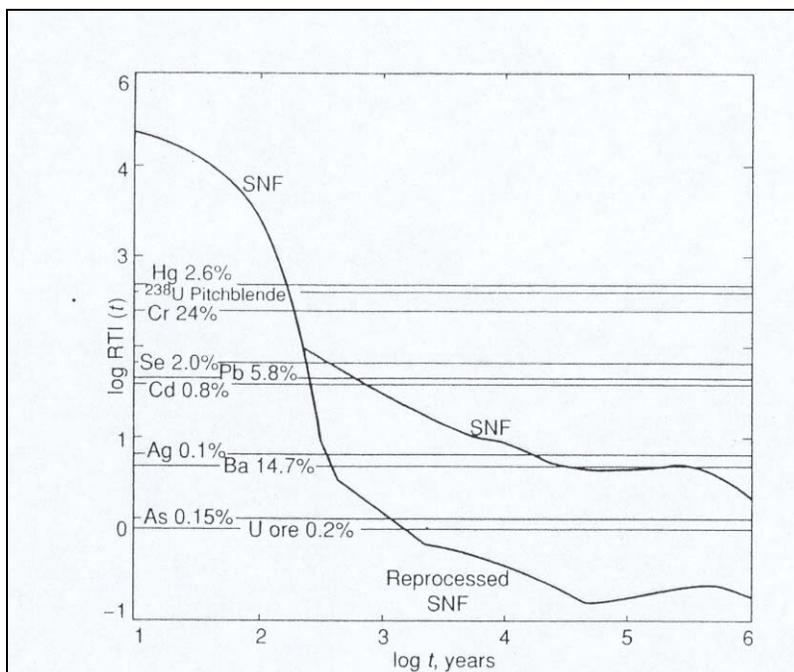
Fig.10. Relative toxicity of selected materials as a function of time<sup>1</sup> (SNF=spent nuclear fuel).
